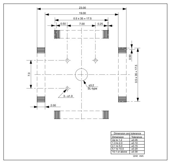
Figure 6 Recommended Dimensions for Mount Pad
